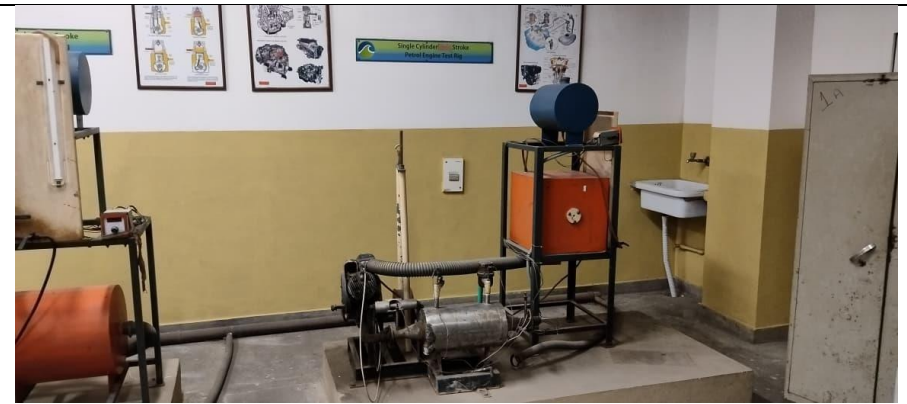
P-14 | C.S.M. of 1-Cyl. 2-Stroke Petrol Engine Date: 25-04-2026 | Geotag: NOT AVAILABLE (no GPS EXIF)
